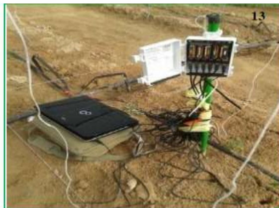
Figure (5): Installing sensors used in scheduling irrigation in one of the greenhouse fields
