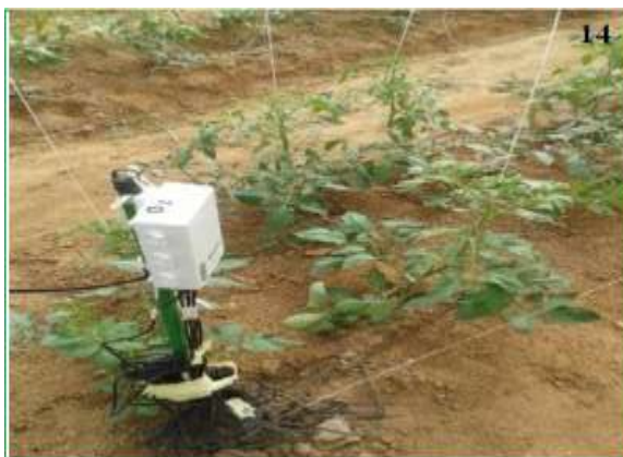
Figure (5): Installing sensors used in scheduling irrigation in one of the greenhouse fields
