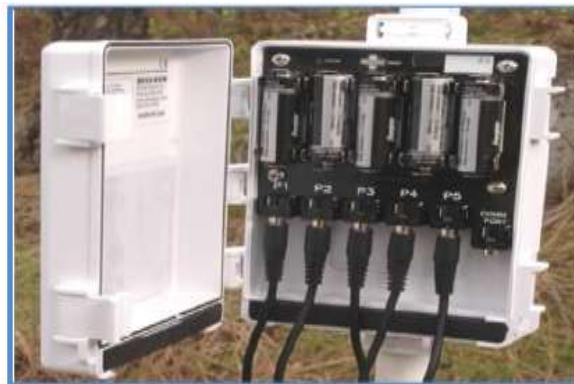
Figure (4): Em50 Data logger manufactured by the American company Decagon Devices
