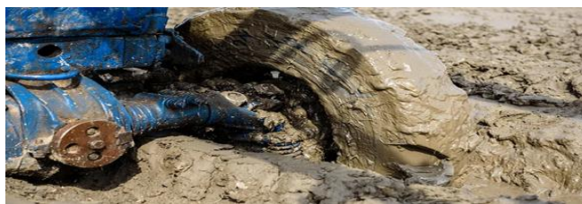
Fig. 4. Stuck tire tractor in saturated clay soil.
