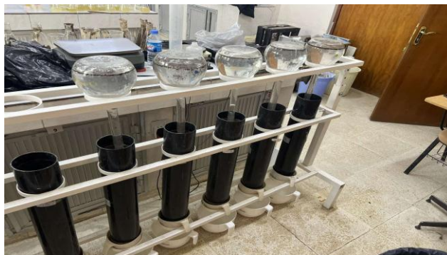
Figure 1: Constant Head Permeameter Apparatus used for measuring hydraulic conductivity ( K_s )
